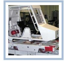
Combustion tractor is compound of: engine part, drive vehicle, brake vehicle, main cabine and auxiliary cabine.
